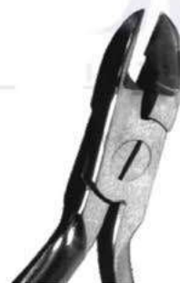
Hard wire cutter 13 cm / 5" 786-2109 Box Joint 786-2110 Screw Joint 786-2111 L-Key Joint For cutting orthodontic wires for fixed techniques any size. Cuts rectangular wire up to 0.56x0.71mm and round wire up to 0.51mm
