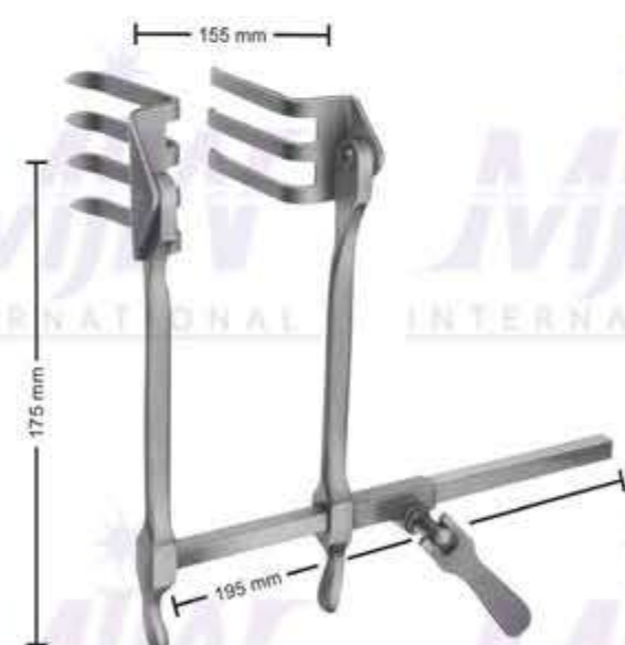
12-468 SCOVILLE-RICHTER Retractor (12-468A) with 1 pair blades (12-469) reversible type. The Retractor bar and shanks may be easily rotated 180° when blades are in situ.
